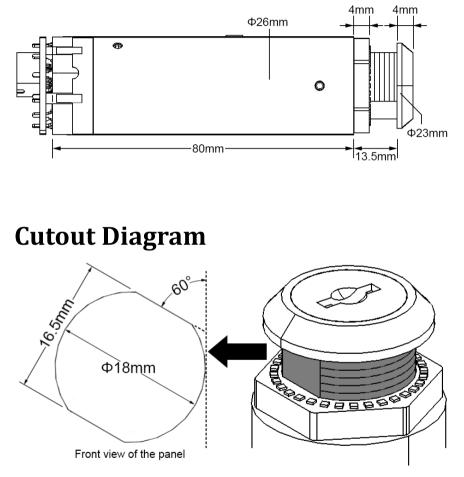
Please be aware that the angle of the flat edge(which is 60° in this diagram) may vary due to different batches of the lock. Please confirm this angle according the actual key switch in your hand before you make the cutout.
