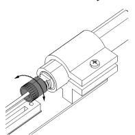
Tighten or loosen the friction nut to adjust friction.
